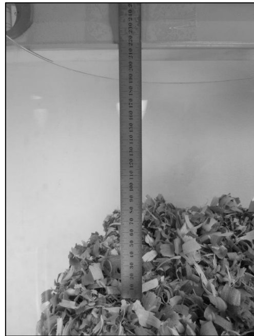
Figure 3-27. Ruler Shown with the Zero End at the Bedding Surface.
