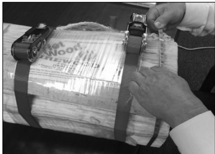
Figure 3-13a. Strapping the Ends of a Bundle.
