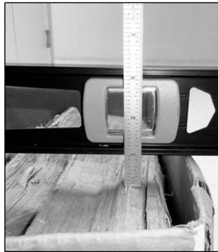
Figure 3-9a. Examples of the Headspace Measurement.
