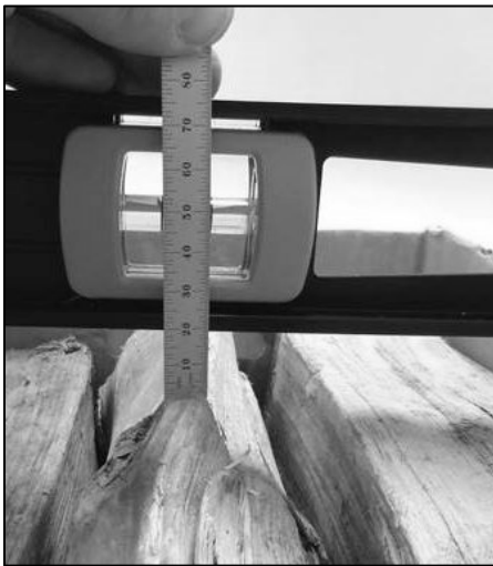
Figure 3-9a. Examples of the Headspace Measurement.
